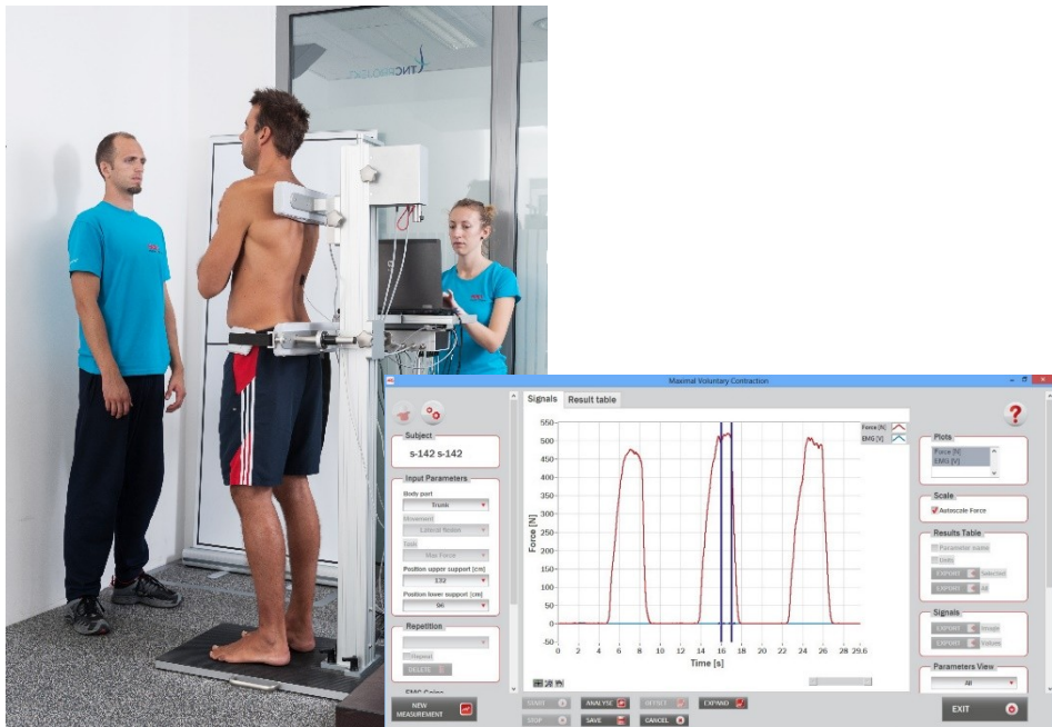
Figure 1: Testing maximal voluntary contraction force/torque for trunk extensors under isometric conditions (left) and the corresponding signals (right).
